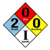
NFPA Hazard Identification system utilizes a four color diamond label and 0-4 numerical hazard rating. The Diamond has an area for health hazards (blue) and area for flammability hazards (red), an area for reactivity hazards (yellow), and an area for special hazard notations.
